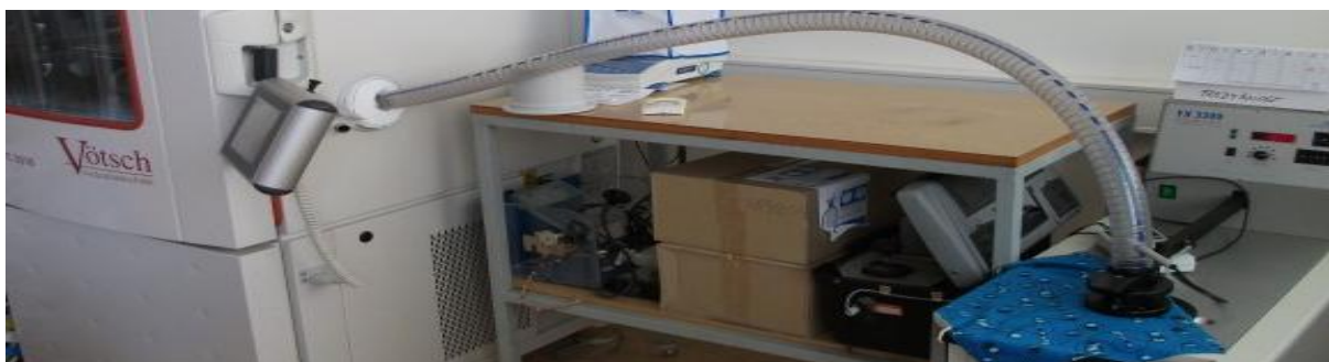
Figure 5. Measuring setup: the source of hot and humid air VOETSCH, air permeability tester FX 3300 and the air temperature and humidity measuring system AHLBORN.
